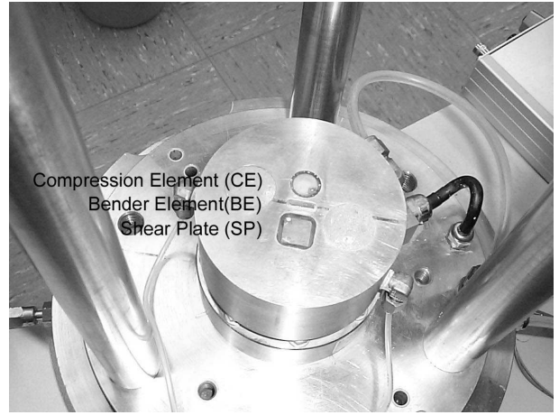
Fig. 2: Photo of piezoelectric elements in the lower specimen end plate
